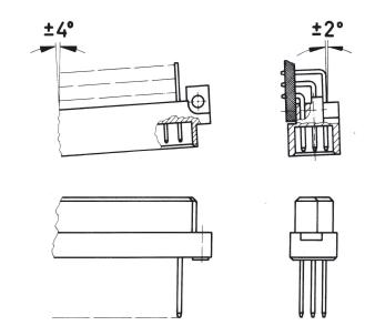
To ensure reliable connections and prevent unnecessary damage, please refer to the application data diagrams. These recommendations are set out in IEC 60603-2.
