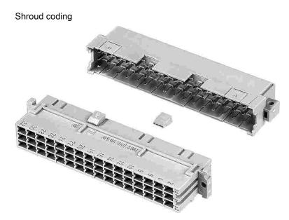
Insert the code key into one of the key ways of the female connector as shown in the drawing. Break out the corresponding area of the male shroud. Connectors coded this way can only be applied in a minimum rack spacing of 20.32 mm.
